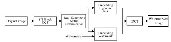
Figure 1. Block diagram of proposed digital watermark embedding system.
