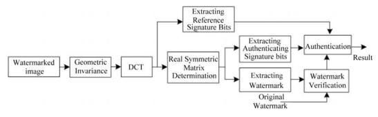
Figure 2. Block diagram of proposed digital watermark extraction system.
